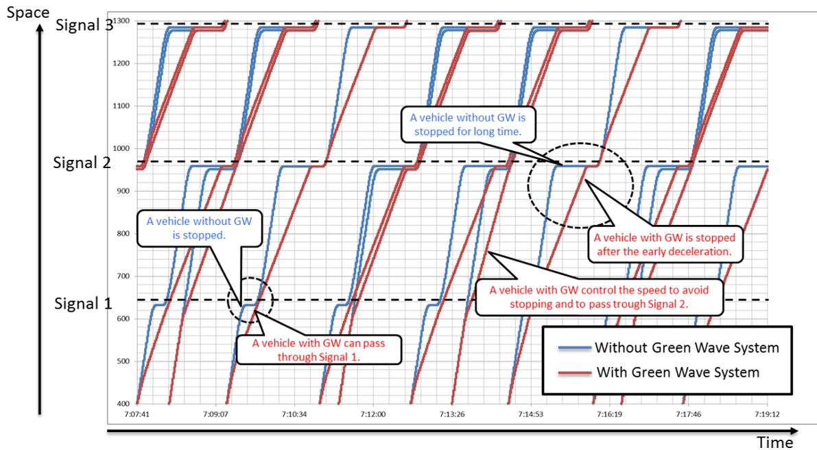
Figure 4 – Demonstration of Green Wave System for Verification
