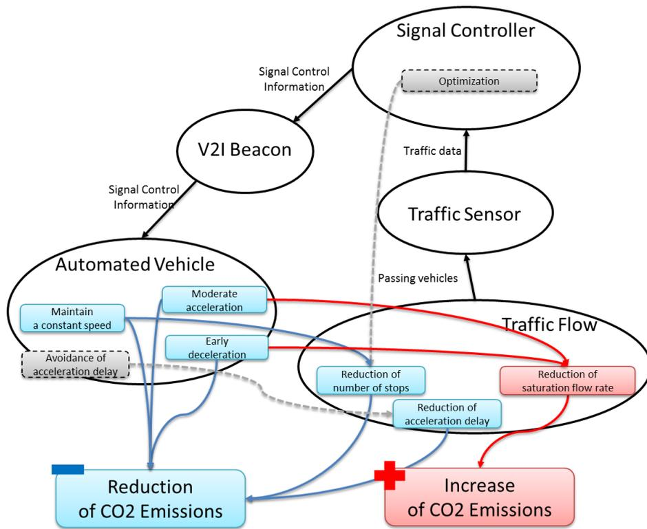
**Figure 2 – Reference Model of Green Wave System with Automated Vehicle**
