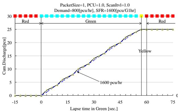
**Figure 16: Link discharging profile at a signal intersection -- SOUND/A-21**
