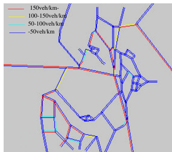
Fig. 4.10. Vehicle Density at 30 min. After the Earthquake
