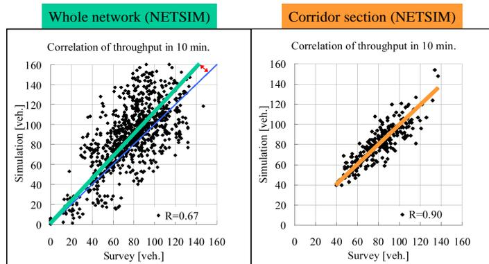
Figure 18: Link Throughput Reproducibility in the Validation of NETSIM [Sawa and Yamamoto. 2002]
