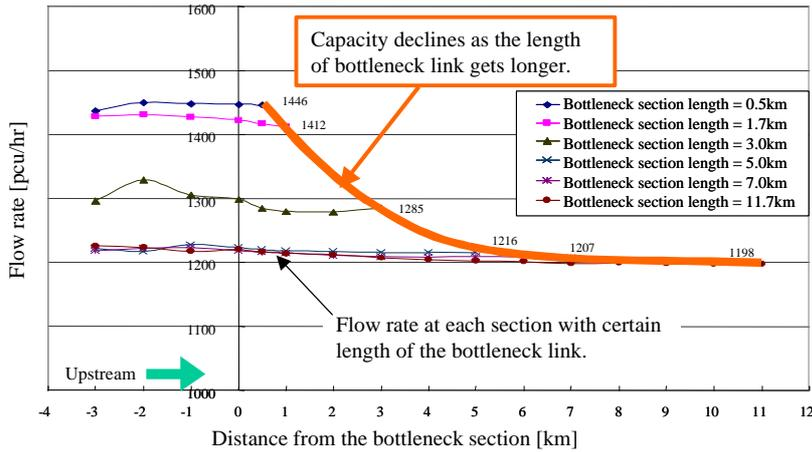
**Figure 15: The capacity varying with the length of bottleneck section (SIPA)**
