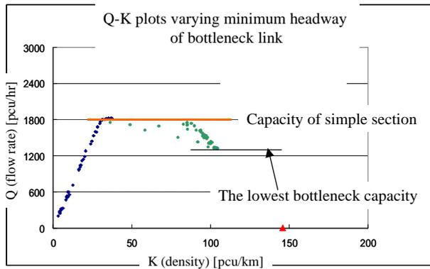
**Figure 14: Bottleneck capacity and traffic flow characteristics of SIPA**
