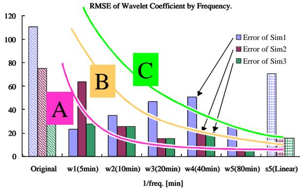
**Figure 23: RMSE of Each Wavelet Coefficient Vectors at Each Frequency.**
