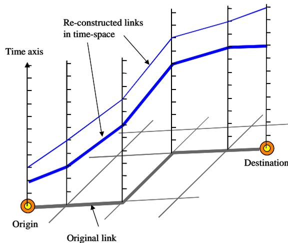
**Figure 19: Re-constructed Time-Space Network Used for OD Estimation [Oneyama, *et al.* 1996]**
