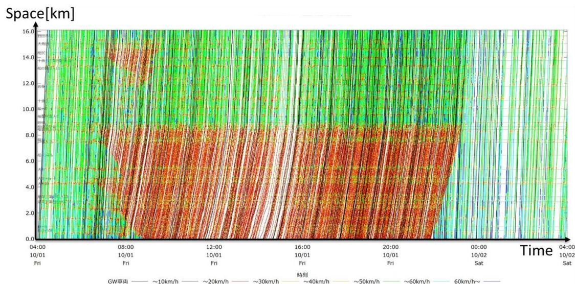
**Figure 7 – An Example of Vehicle Trajectories of Base Case (without GW), from South to North**
