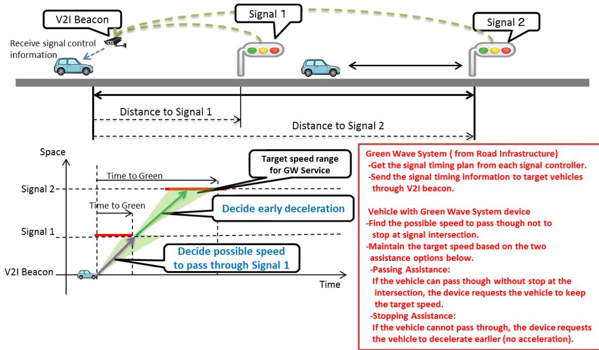
Figure 3 –Implemented model of green wave system
