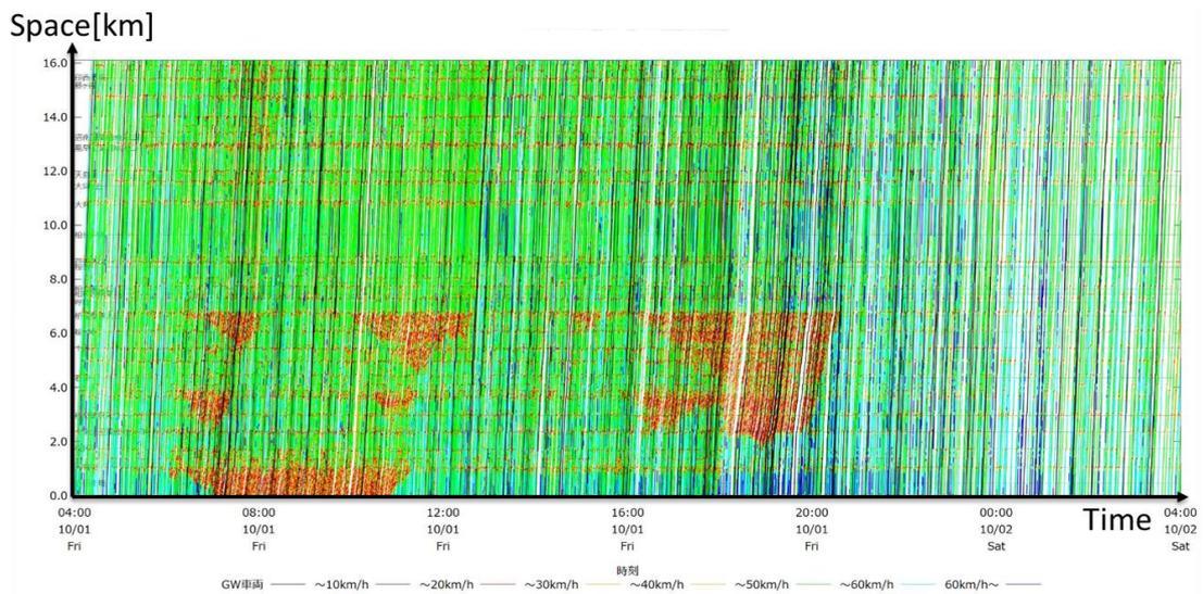
Figure 6 – An Example of Vehicle Trajectories of Base Case (without GW), from North to South
