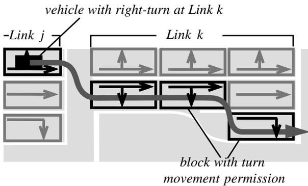
Figure 4: The modelling of the lane choice behavior in the Hybrid Block Density Method
