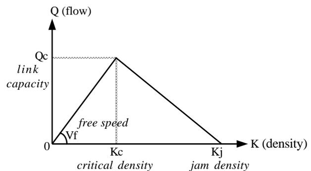
Figure 1: The flow-density relationship used in the Block Density Method
