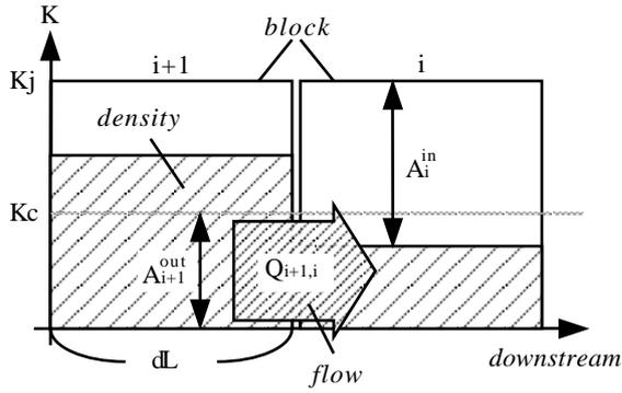
Figure 2: The flow calculation between two neighboring blocks
