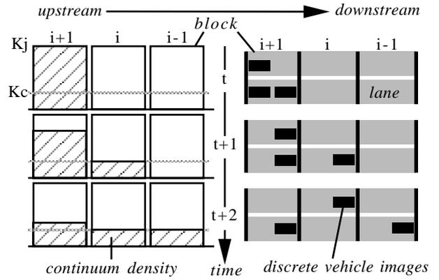
Figure 3: The movements of discrete vehicles in the Hybrid Block Density Method
